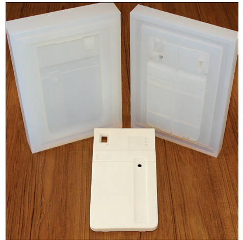
RTV Rubber Mold and Urethane Cast Part.
